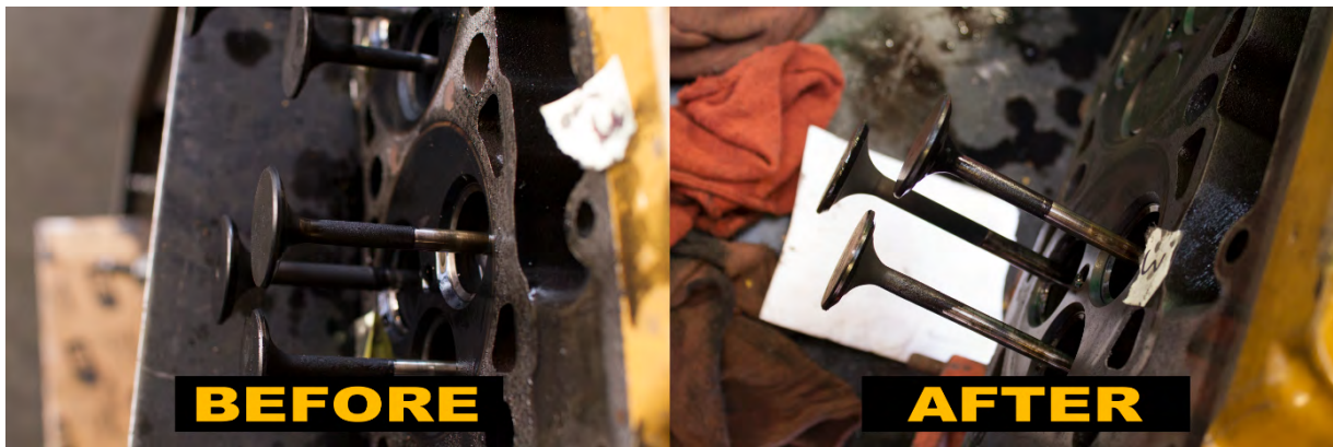
Figure 3-4. Before and After Pictures of Valve Stems.
