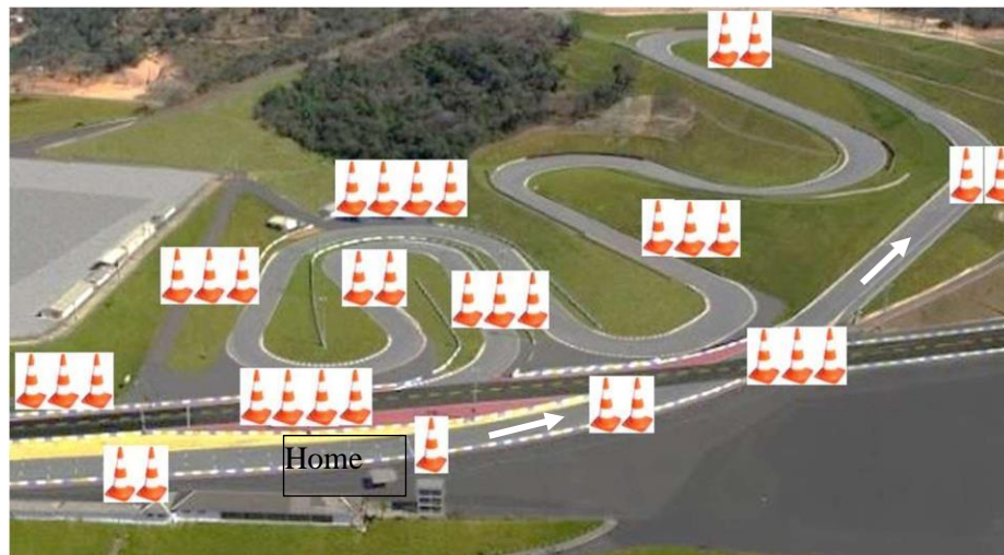
Figure 1: Aerial view of the track used for measuring consumption and indication of the exchange points and inserted gear (cones).
